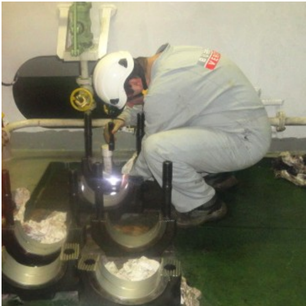
Bearing Shell inspection
