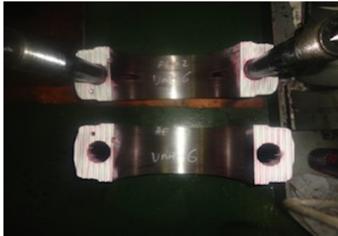
DP test for big end halves
