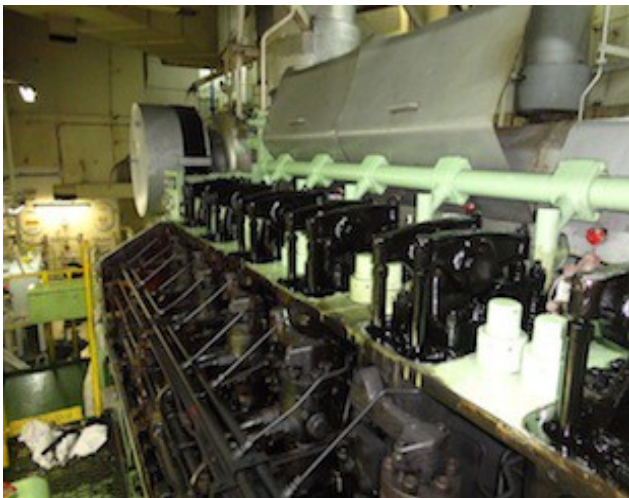
Opening Marine Generator for D'carb
