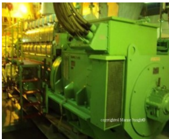
Alternator connected to bus bars
