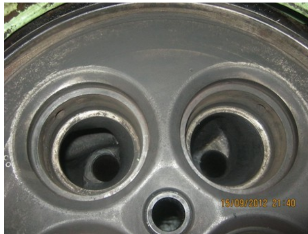
Valve seat corrosion & Scoring
