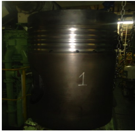
Cleaned Piston and ring groove
