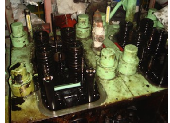
Removing all connections from Head
