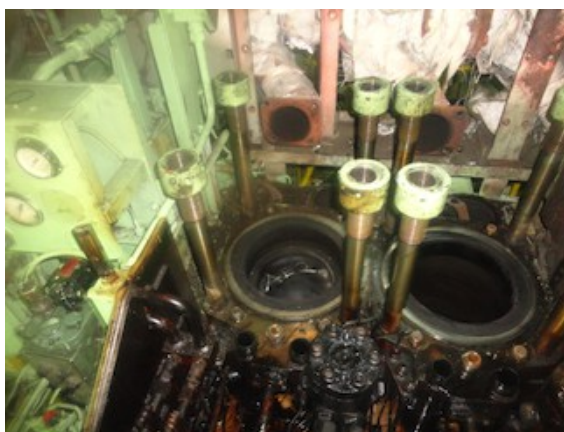
Protect Head stud threads by putting back nuts
