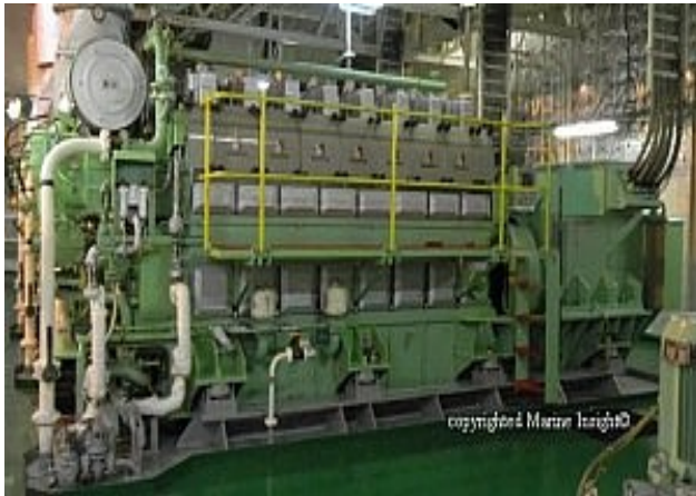
Generator- Prime mover & Alternator
