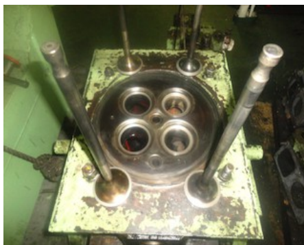
Valve and Seat after lapping
